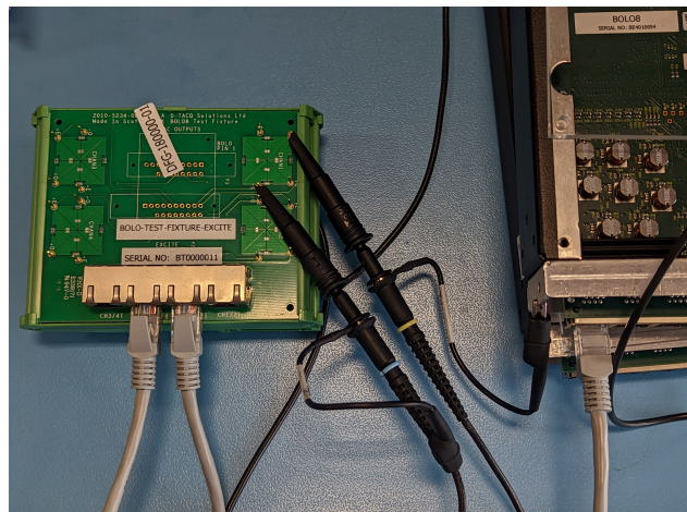
(b) Probes on EX+ and EX- measuring output from Excite DAC
