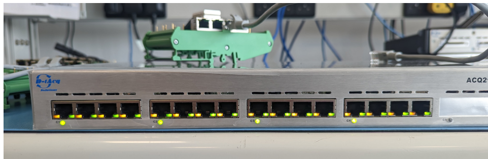
Figure 23: Example front panel showing B8 Mezzanine RJ45 LEDs
